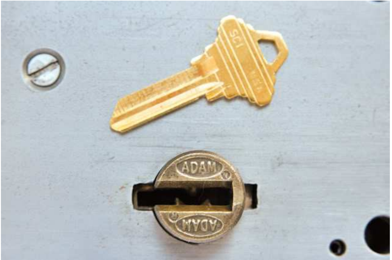
Similar to a number of safe locks, the bolt is drilled and tapped, and can have other boltwork mechanisms attached to it:
